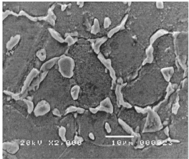
Figure 4 Carbide precipitate in Inconel 718 base metal.
